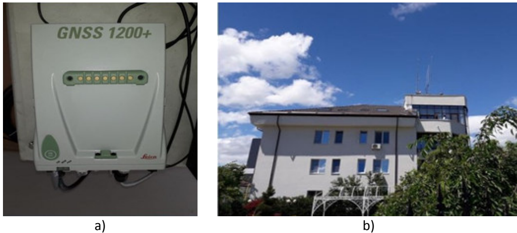
Fig. 4. The GNSS technology used in research: a) the GNSS receiver Leica 1200+; b) reference station CRA
