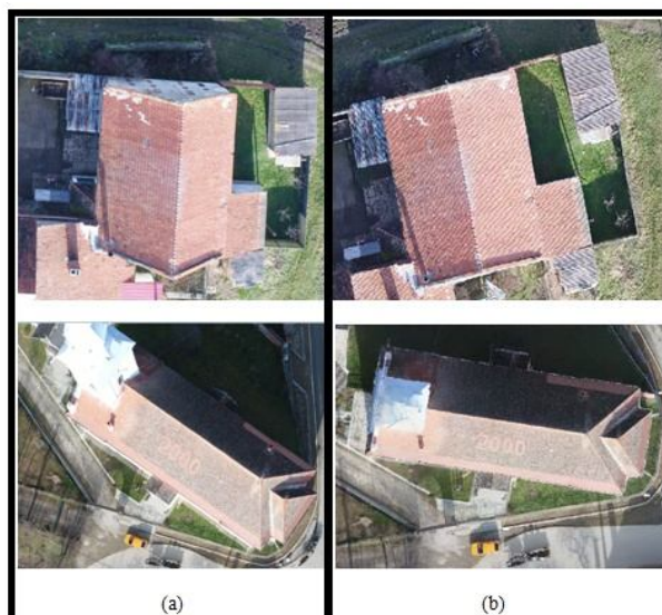
Fig. 7. Raw images in which can be seen lateral view of details (a) and orthorectified images based on DSM (b)
