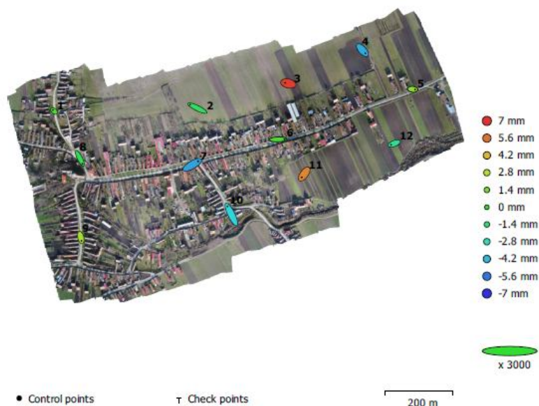
Fig. 6. GCP location and error estimates Z error is represented by ellipse color. X, Y errors are represented by ellipse shape
