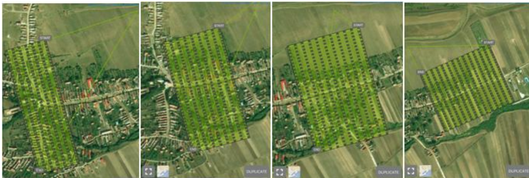
Fig. 2. Flight plans made with PIX 4Dsoftware as four photogrammetric blocks
