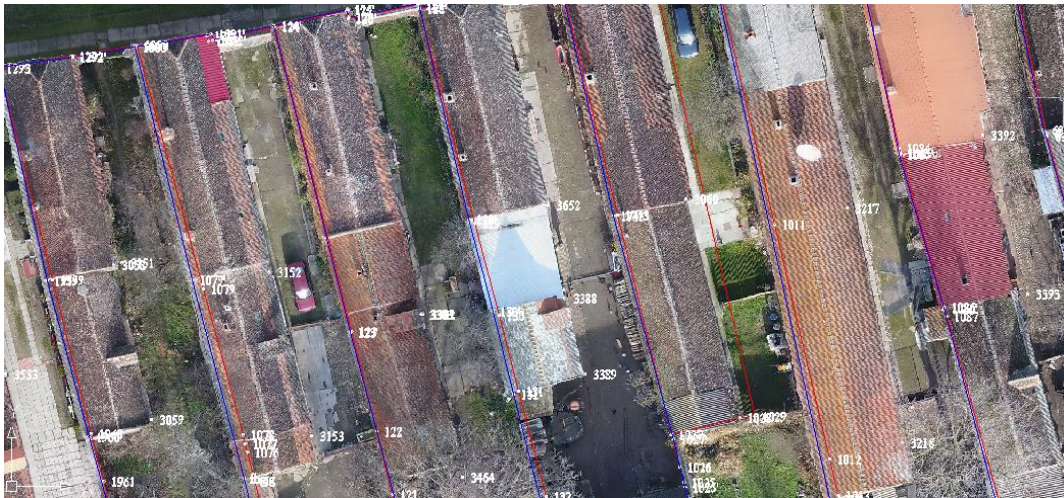
Figure 5. Part of the orthophotomap vectorized: red color-official limit of ANCPI (e terra 3); blue color-vectorized limit based on the orthophotomap made based on the images received with the UAV
