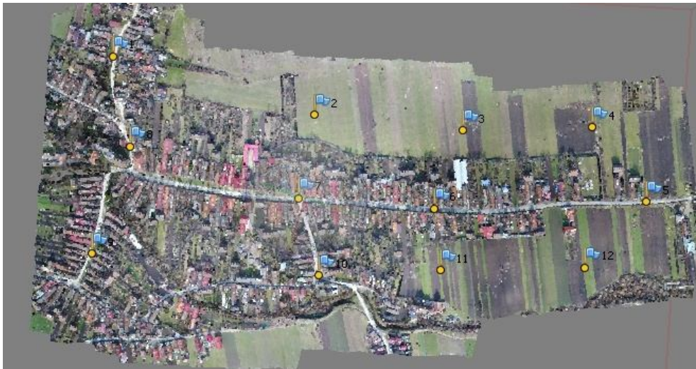
Fig. 4. Dense point cloud and distribution of photogrammetric marks within the studies area
