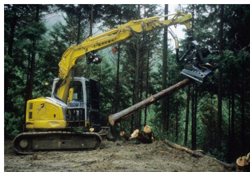
Fig. 4. A typical harvester mounted on excavator at roadside equipped with a small winch for prehauling (Photo: Hideo Sakai)
