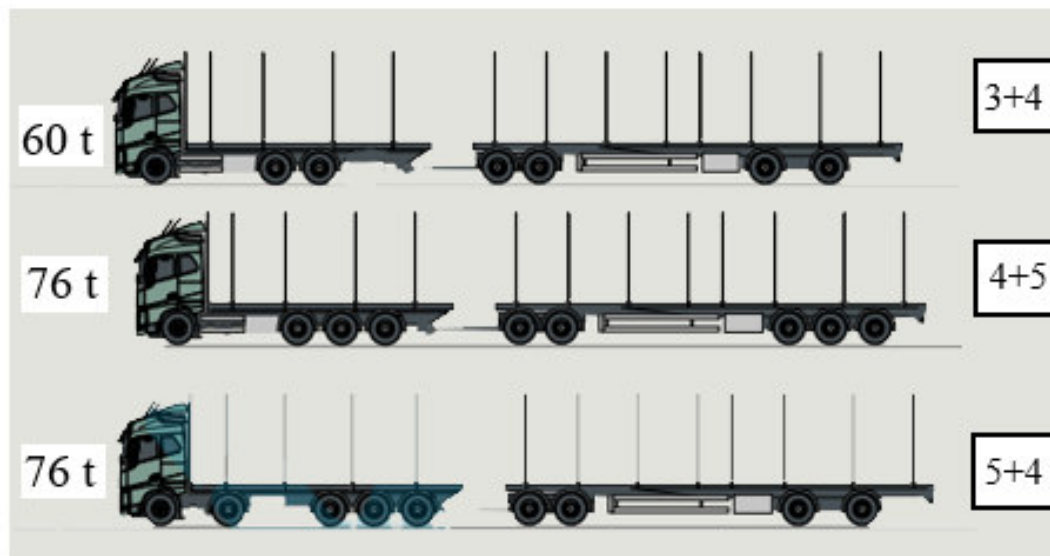
Fig. 1. Most common axle solutions of timber transport vehicle combinations (60 and 76 t)
