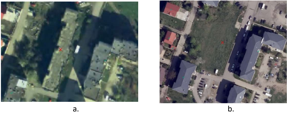
Fig. 10. Identifying demolished buildings: a. orthophoto 2012; b. orthophoto 2022
