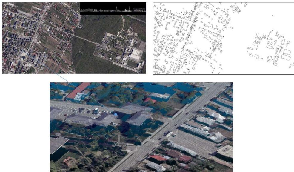
Fig. 4. Input datasets: photogrammetric point cloud and building footprints
