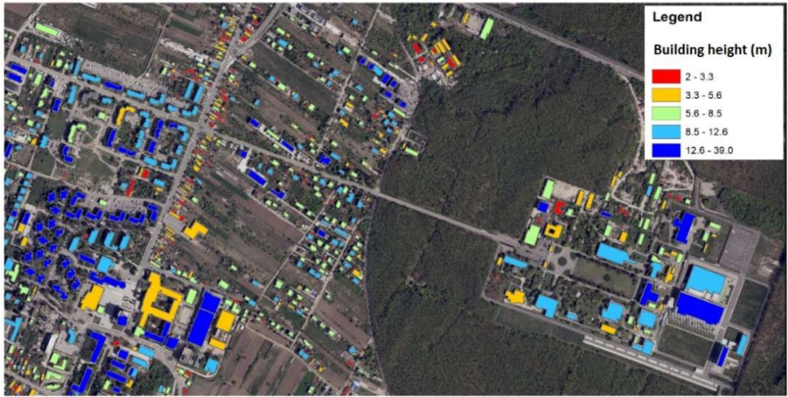
Fig. 8. Building footprints highlighted by the height value
